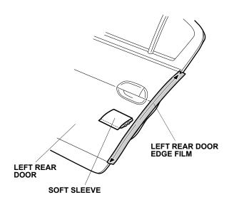
20. Carefully remove the outer protective film from the left rear door edge film.
