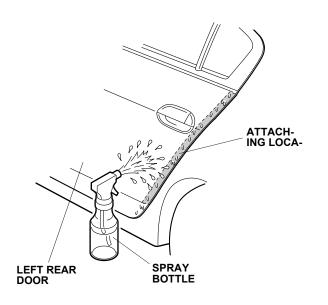
19. Starting from the center and working outward, use the soft sleeve to smooth out the left rear door edge film. Move the applicator in only one direction.
