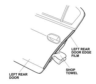
23. Repeat steps 1 through 22 to install the door edge film on the right side of the vehicle.
