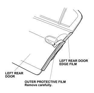
21. Starting from the center and working outward, fold the left rear door edge film around the left rear door edge. Be careful not to damage the door seal during this procedure.
