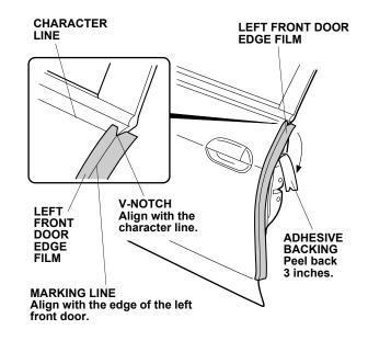
7. When the alignment is correct, apply light pressure to the door edge film while you carefully remove the adhesive backing. Don't worry about wrapping the door edge film around the door at this time.
